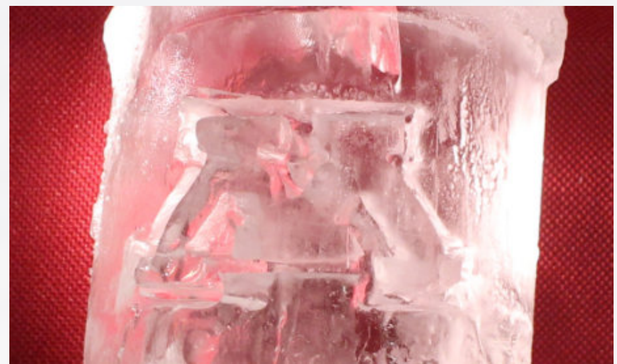
Wedge cut from 3" diameter tap-water core using 1.07 \mu\text{m} laser (250 W)
