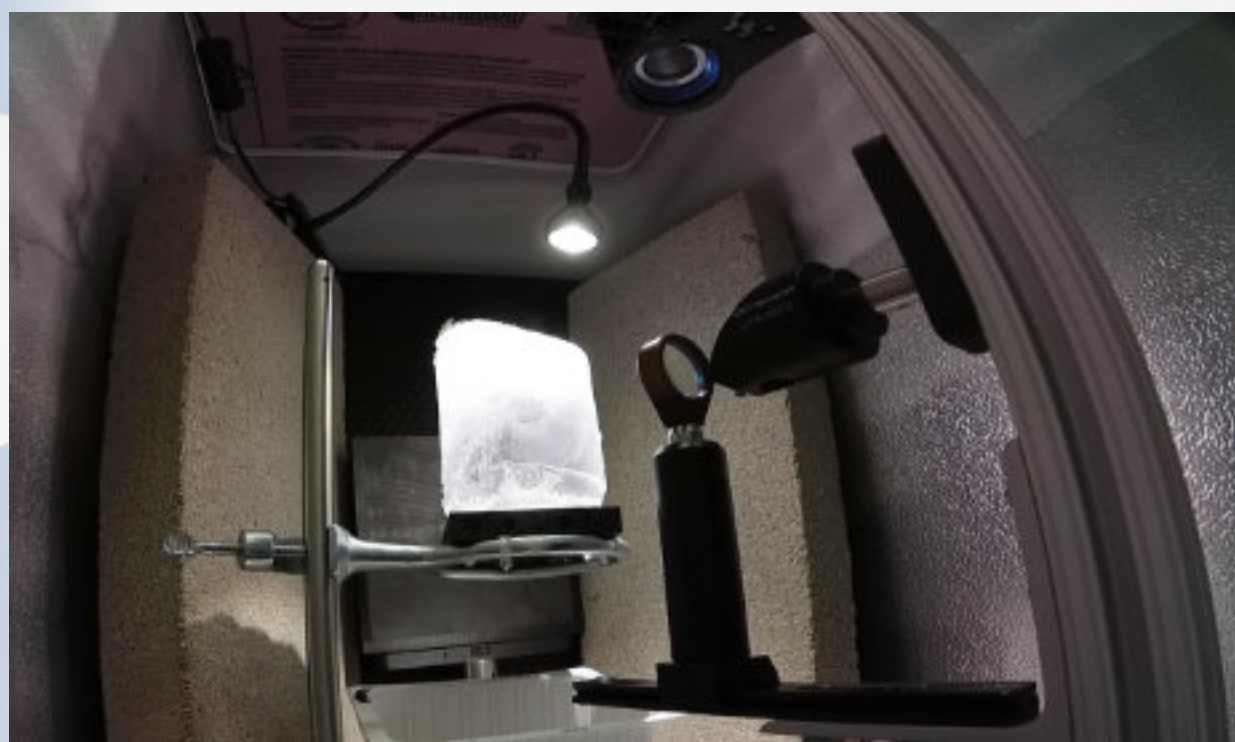
Fisheye photo of a basic laser-cutting motion setup at work inside lab freezer
