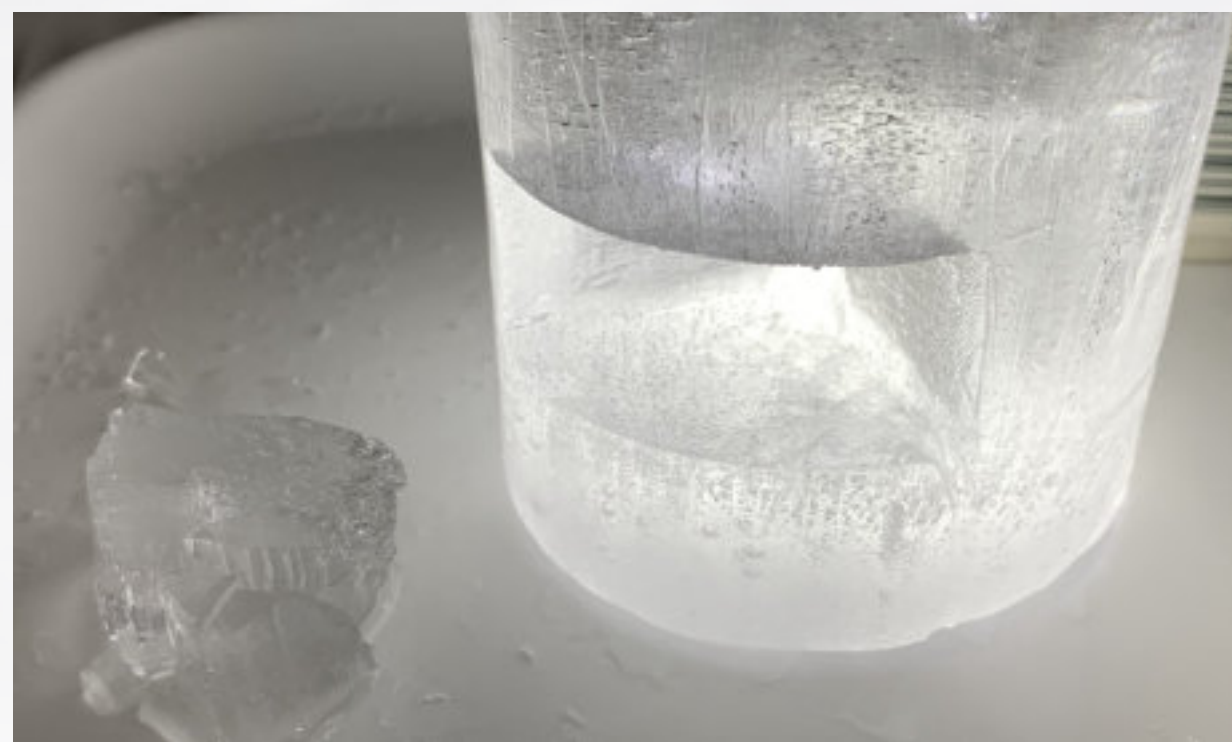
Wedge cut from 3" diameter tap-water core using 1.07 \mu\text{m} laser (90 W)
